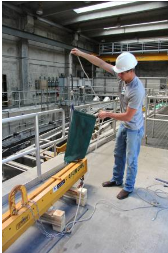
Figure 2. Fish net attached to pulley on beam.
